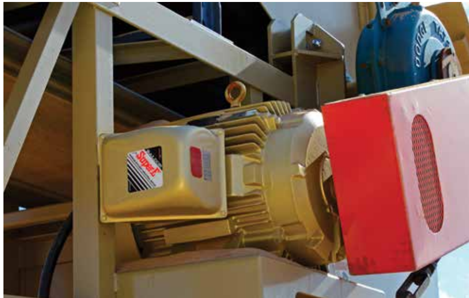
Baldor•Reliance Super-E® premium efficient motors and Baldor•Dodge Torque-Arm II gear reducers, chosen because of their superior performance and reliability, power the 21 grasshopper conveyors supplied for the El Castillo project.
