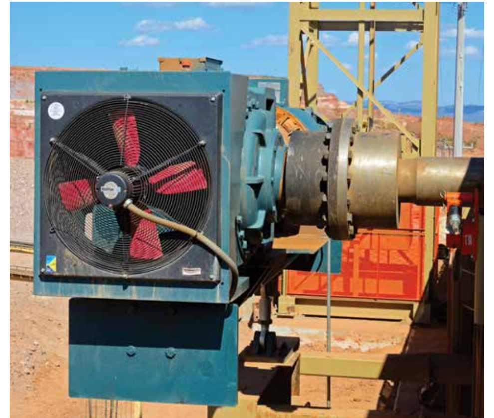
This Dodge DM Moment coupling is specifically designed to make the rigid connection between the output shaft of the gearbox and the head pulley. Custom-engineered for each application, the DM Moment coupling is capable of handling both the torque and the bending moment forces of the suspended weight of the drive package, including the gearbox, motor, fluid coupling and swing base. This design also allows for an alignment-free drive by eliminating the time-consuming process of aligning the gearbox assembly to the head pulley shaft.
