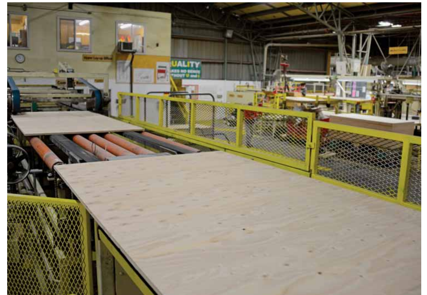
Baldor's Dodge Quantis reducers help power the newly built equipment that ties the poly line, the panel turner and the sanding line into one continuous process.
