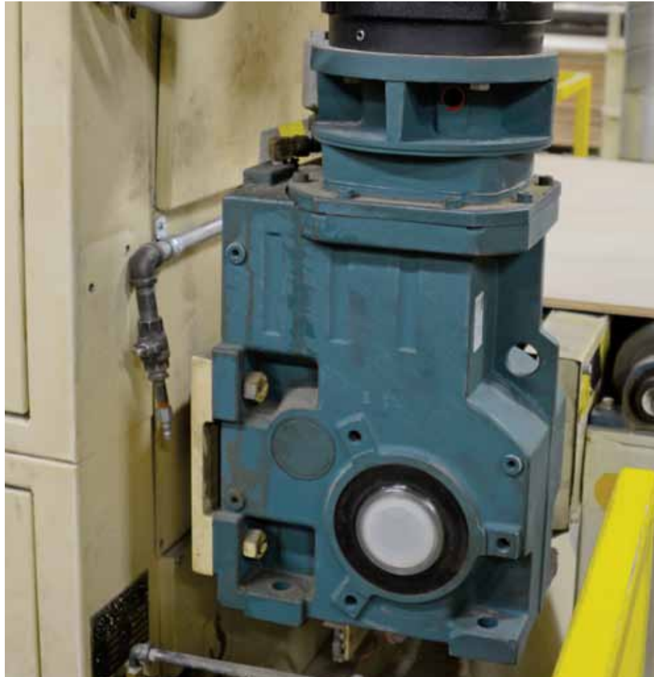
This size 108 RHB Quantis reducer replaced a competitor's gearbox so operators can better control the speed of the transfer belts on a sanding machine. Some wood panels need to be sanded quickly while others need to be sanded more slowly. With the Quantis gearbox installed, operators can now utilize the full speed range of the sander.
