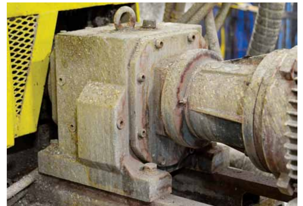
Lead Millwright Chris Stevens says he knows from experience that Dodge Quantis units are rugged and reliable. The proof, he says, is this Quantis ILH unit on a roll coater machine, one of the toughest applications in the mill. Despite the shock load and machine vibration, which has cracked the feet of other gearboxes, this Quantis reducer has performed without a problem for the past eight years.
