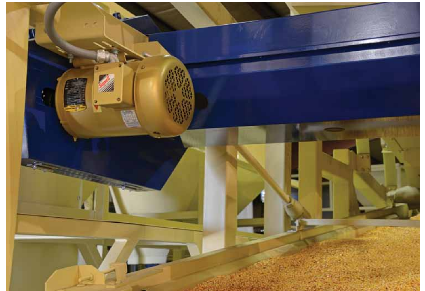
Product quality and reliability was another factor that convinced LMC to choose Baldor as its global partner. This Baldor•Reliance Super-E® motor is powering a vibrating conveyor that is sizing popping corn.
