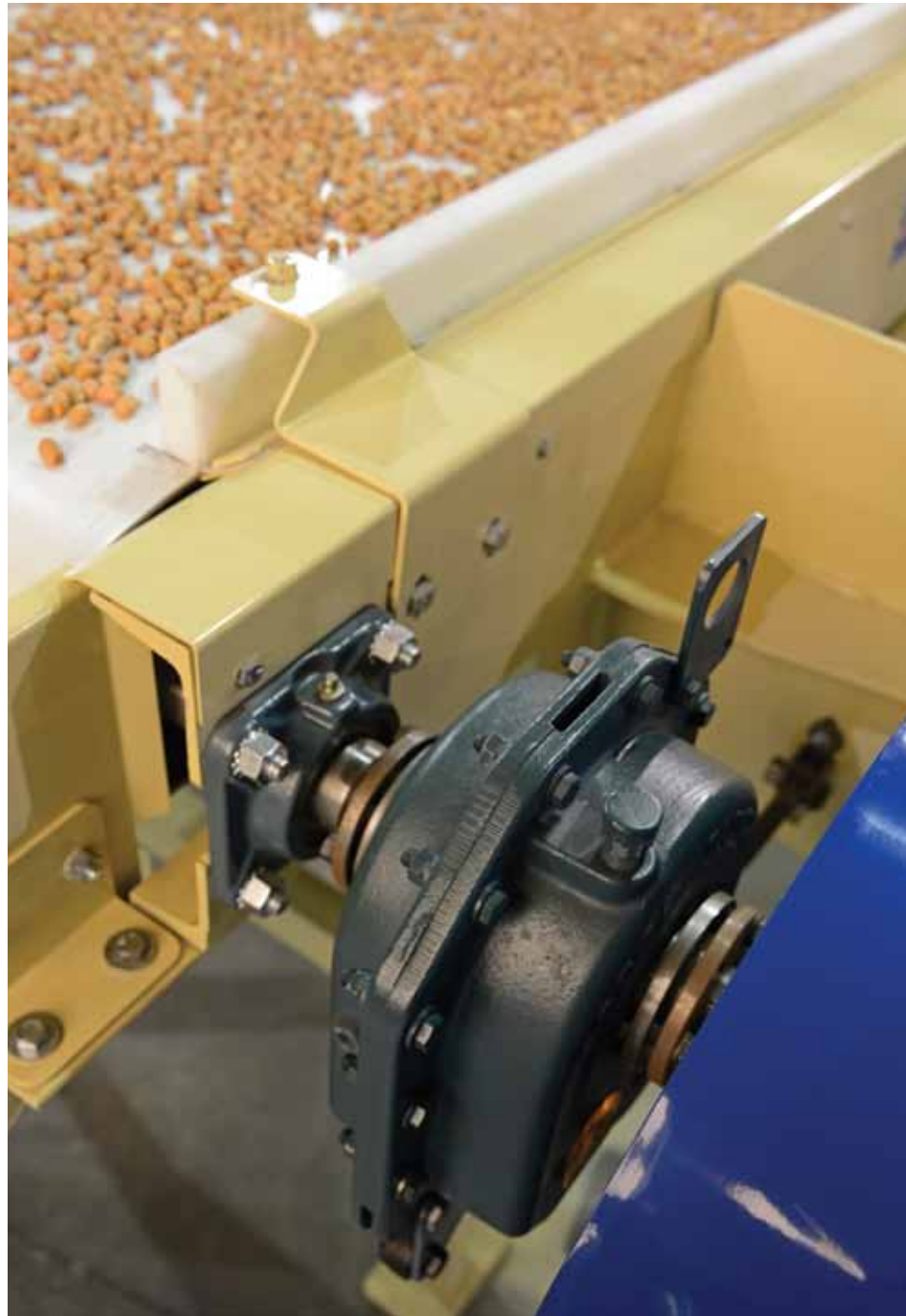
Today, 100 percent of the peanut crop in the U.S. is processed by LMC equipment, like this picking conveyor featuring Baldor's Dodge Torque-Arm II™ reducer and Dodge bearings. Currently 60 percent of LMC's business is export, but with proven technology and Baldor as its global partner, LMC is prepared for major growth around the world.
