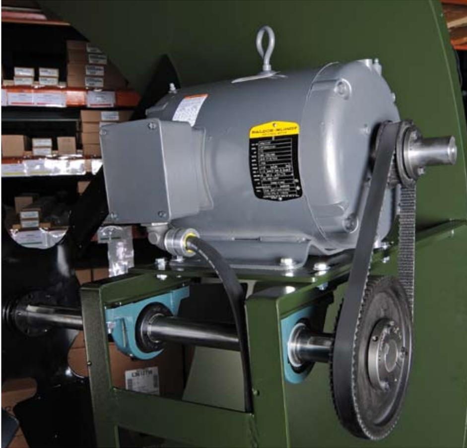
TurfBreeze fans are made of steel, with a strong powdered coating to withstand the elements. Inside you'll find what TurfBreeze officials describe as premium products: a Baldor•Reliance motor and Baldor•Dodge mounted ball bearings and synchronous belt drive.
