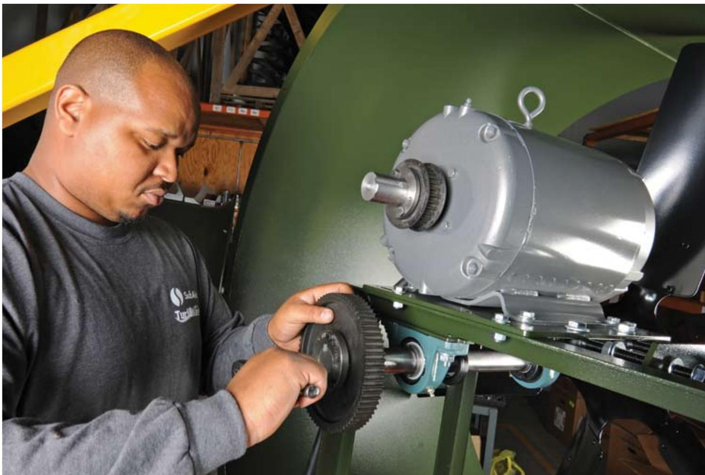
Switching from V-belts to the Baldor•Dodge synchronized drive system means there is no maintenance required after installation. The synchronized sprockets are coated with black oxide to prevent rust. This synchronized system is also more energy efficient and has allowed TurfBreeze to optimize fan performance.
