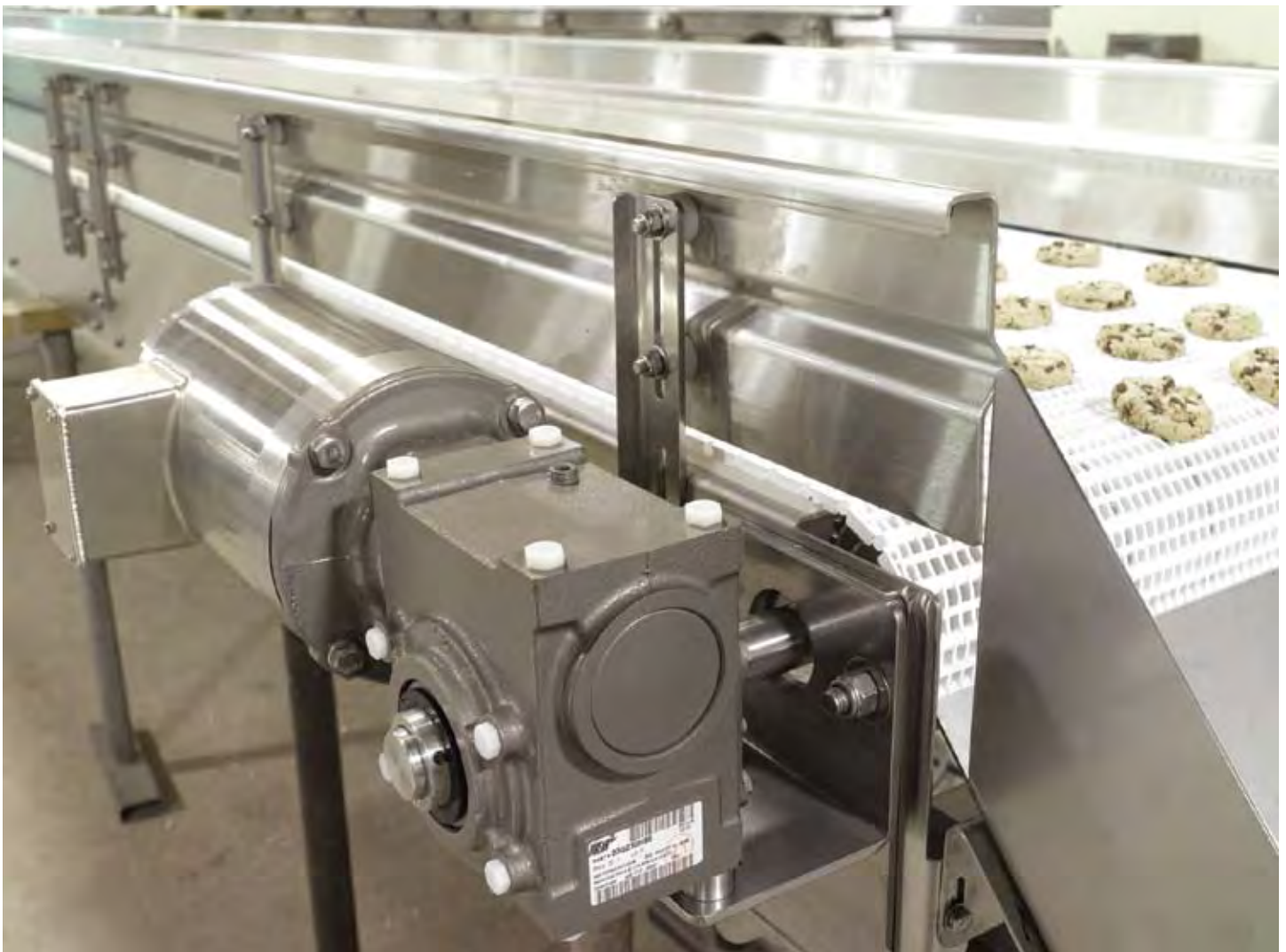
Nercon selected Baldor® Reliance Super-E Stainless Steel Encapsulated motors and Baldor® Dodge EZ Kleen Tigear-2 reducers for this washdown application because these products will last longer under frequent high-pressure sanitizing with caustic chemicals.
